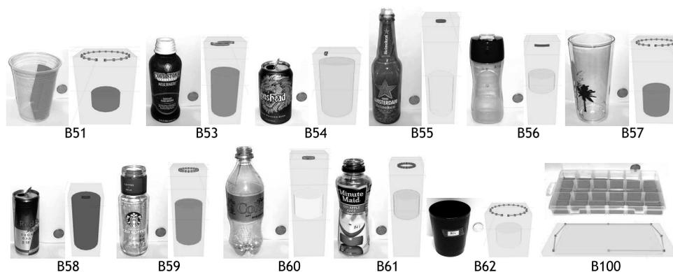
Fig. 18. Containers and their models. Each model has a graspable cylinder, a polygon of the mouth, and the bounding box. The mouths of the containers B54, B56, and B58 are not located at the center.
