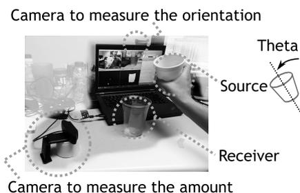
Fig. 2. Setup to measure a human demonstration.
