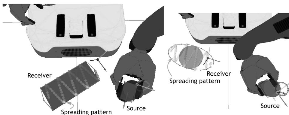
Fig. 20. Planning result of spreading pattern (in simulation).
