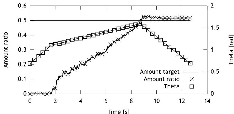
Fig. 11. Typical result of pouring. The setup corresponds to that of the human demonstration (Fig. 3); the source container is B1, and the poured material is the dried peas. For the consistency with Fig. 3,  $\theta$  (Theta) is shifted so that their ranges match with each other.
