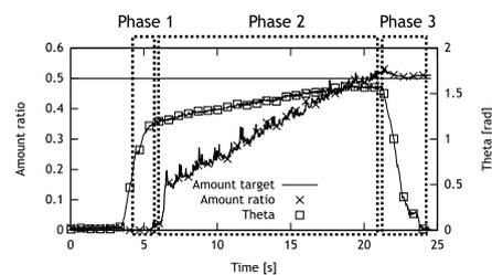
Fig. 3. Result of a human demonstration. The amount trajectory and the orientation (Theta) trajectory are plotted.
